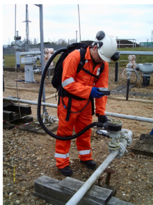
Fig. 2. Example of a sampling method: Bacharach HI FLOW® sampler in operation.
