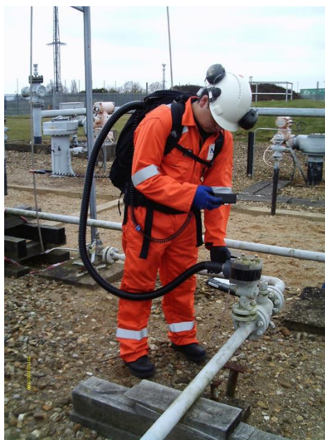
Figure 4. Example of a sampling method: Bacharach Hi Flow® sampler in operation.
