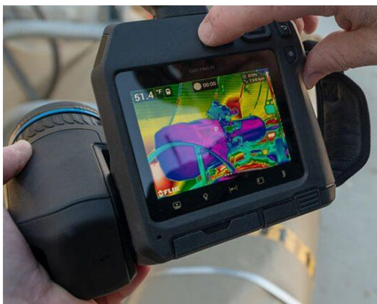
Figure 3. An example of an uncooled and handheld variant of a gas imaging camera.
